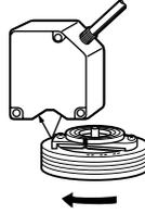
1. Position the sensor head. Be careful about the measuring range and angle of the sensor head.
