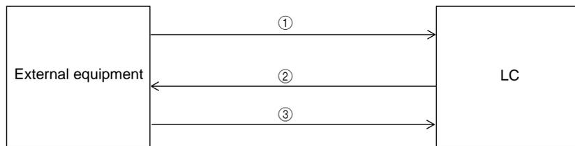
1. Transmit the proper character or ASCII code from the external device to the LC.
